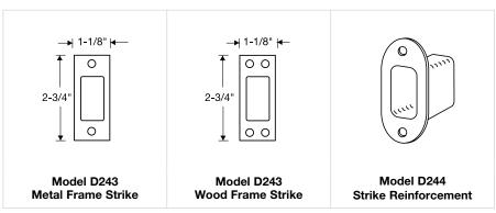
Note: Model D243 is a strike packet which includes both wood and metal frame strikes and corresponding screws.
