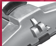
Center Bolt Full 3/4" (19mm) projection, 1" (25mm) wide, positive deadlocking by auxiliary bolt
