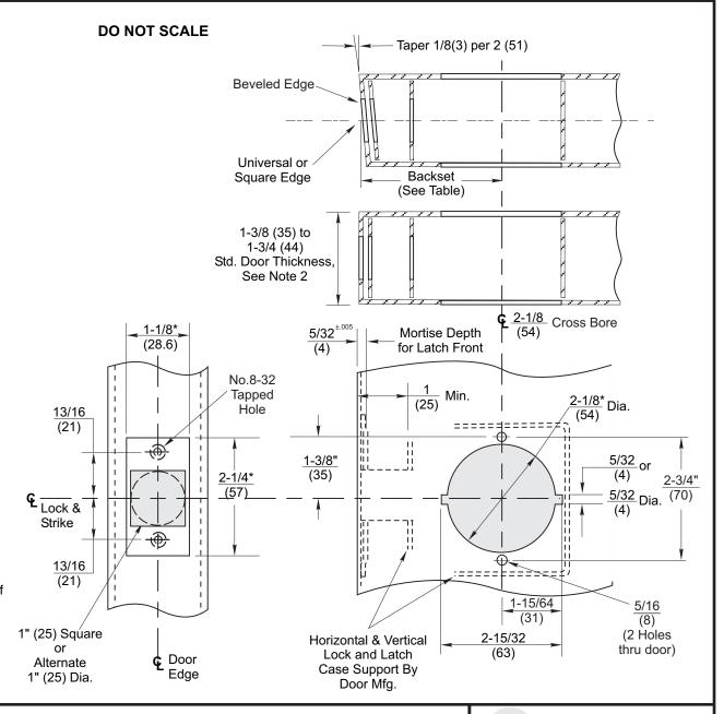
5400LN Series Key-in-Lever Cylindrical Locks - 1-1/8" Wide Front H.M. Door Preparation (See ANSI/BHMA A156.115)
